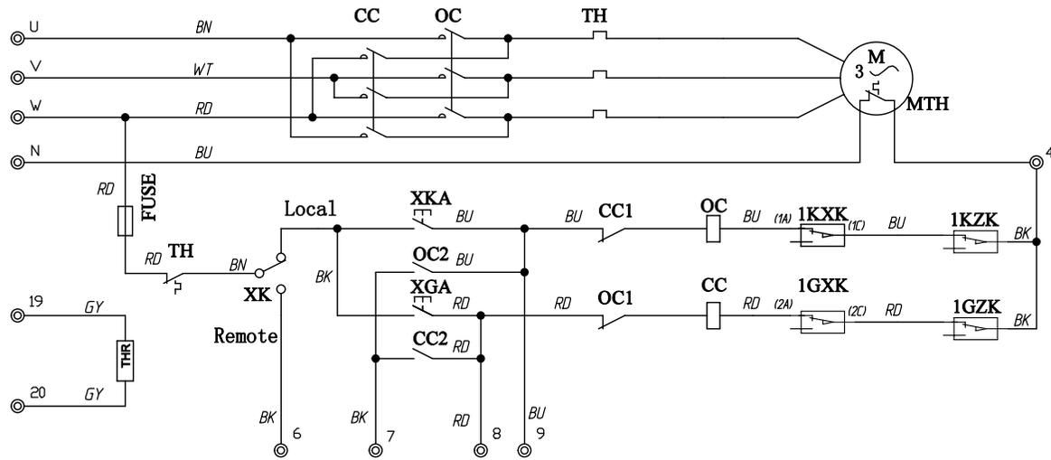
**Limite switch acting procedure**
